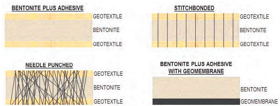
Figure 3-12 Typical GCL cross-sectional configurations (modified from GRI, 2000)
