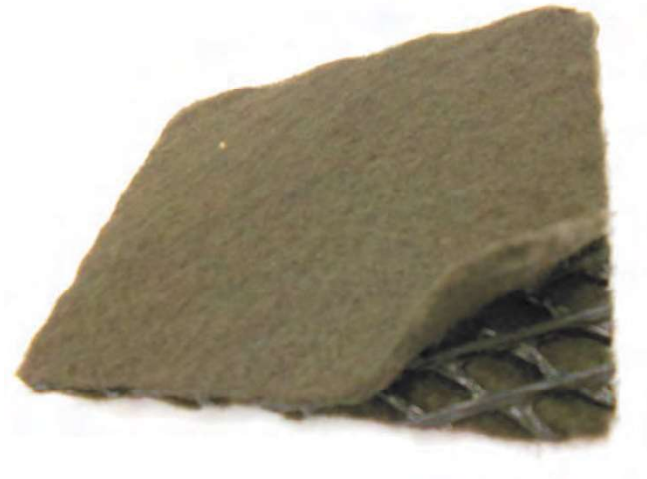
Figure 3-18 Double-sided geocomposite, showing the geonet sandwiched between layers of geotextile
